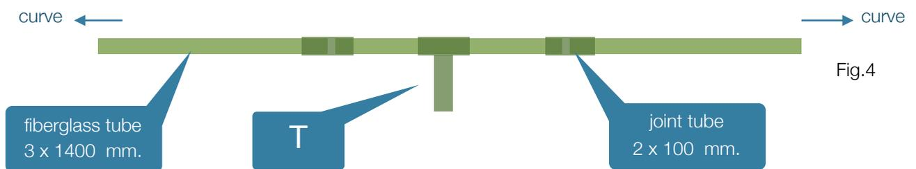
Before joining the three elements with joints you must insert the "T" shaped support.
